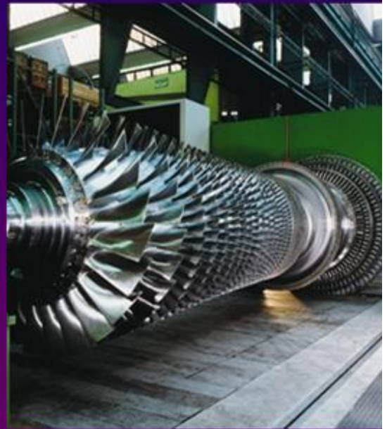
ALSTOM INDUSTRIAL GAS TURBINE ENGINE Alstom = 10% of world IGT market
